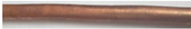
Figure 1. Initial Cu-ETP wire rod with a diameter of 8.5 mm provided by ENICAB
