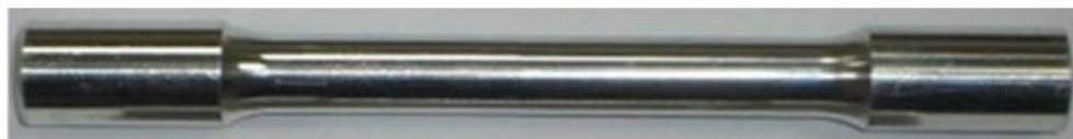
Figure 1. Geometry and dimensions of the standardized cylindrical tensile specimen machined by CNC according to ISO 6892-1.
